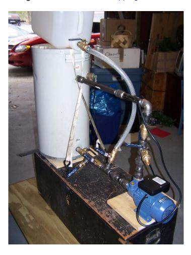
This is the first of two posts about biodiesel; this one explains how to make a biodiesel processor, so you can convert vegetable oil into usable diesel, the second post will actually show how to use the biodiesel processor to make your own biodiesel.
