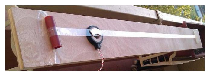
Windbelt is an ultra efficient and mechanically very simple wind generator alternative. Its cheap components can be bought almost anywhere in the world. Windbelt is originally an innovation of mr. Shawn Frayne. He constructed this simple device with a taut Mylar membrane fitted with a pair of Neodymium magnets that oscillate in and out of coils because of the mechanical resonance of the membrane with wind blowing across it. This can be built very easily.
