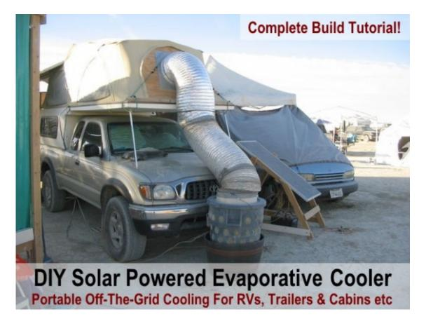
In arid areas of low humidity (desert/ southwest US etc) an evaporation cooler or swamp cooler can reduce the temperature of a room by 20-30 degrees. In many cases they are even more effective than traditional air conditioning. Evaporation coolers are also very low-tech and cheap and easy to build and run. In fact the DIY evaporation cooler in the tutorial below is run via solar power.
